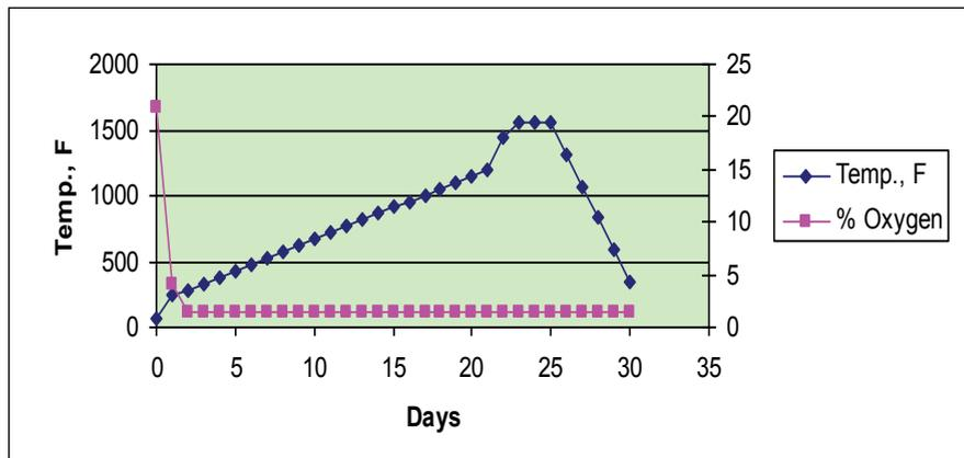
Figure 1. Sample carbon firing cycle.
