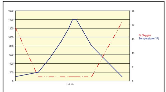
Figure 4. Typical firing curve for carbon-based products.
