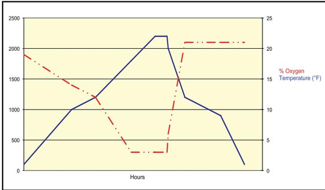
Figure 1. Typical whitewares firing curve.
