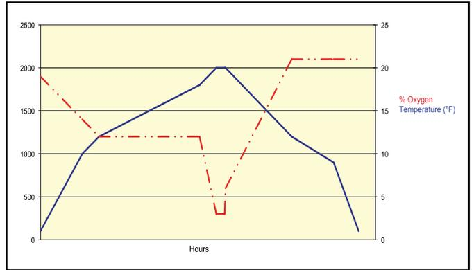
Figure 2. Typical structural clay firing curve.
