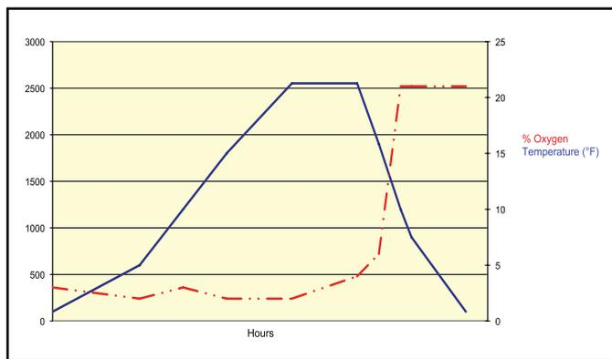
Figure 3. Typical firing curve for specialty ceramics with high binder content.
